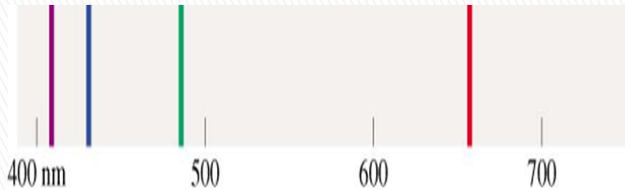
Line Emission Spectrum of Hydrogen Atoms
