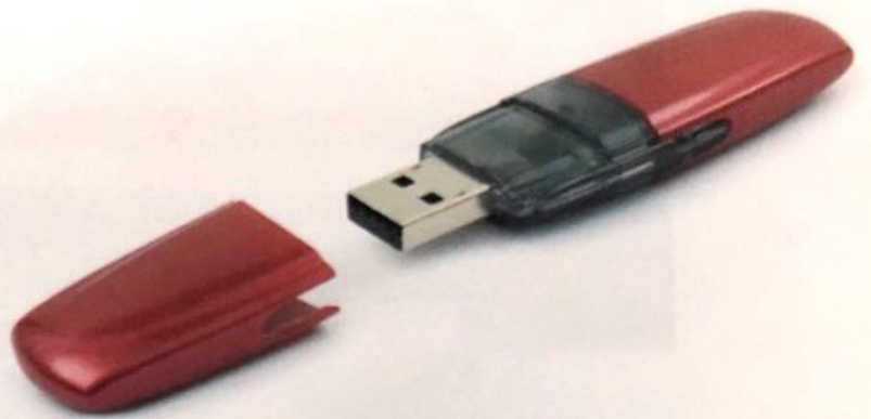
Figure 50 Flash memory devices. a. An SD flash memory card is one of the most popular kinds of solid-state storage used in digital cameras and other digital media devices. b. A USB flash (thumb) drive can store gigabytes of data and plug into a computer's USB port.
