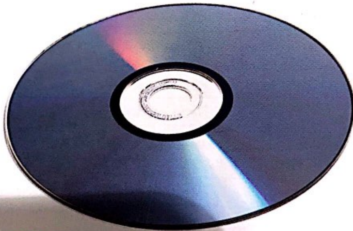
Figure 47 The data on an optical disc is read by a laser.
