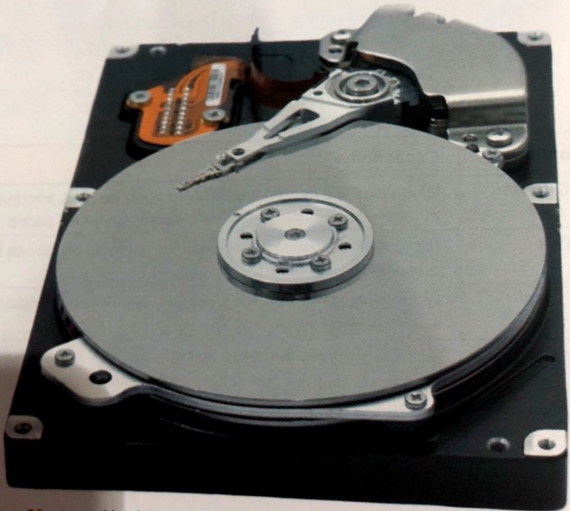
Figure 51 Internal hard drives hold the data and instructions that the computer needs and are inaccessible from outside the system.
