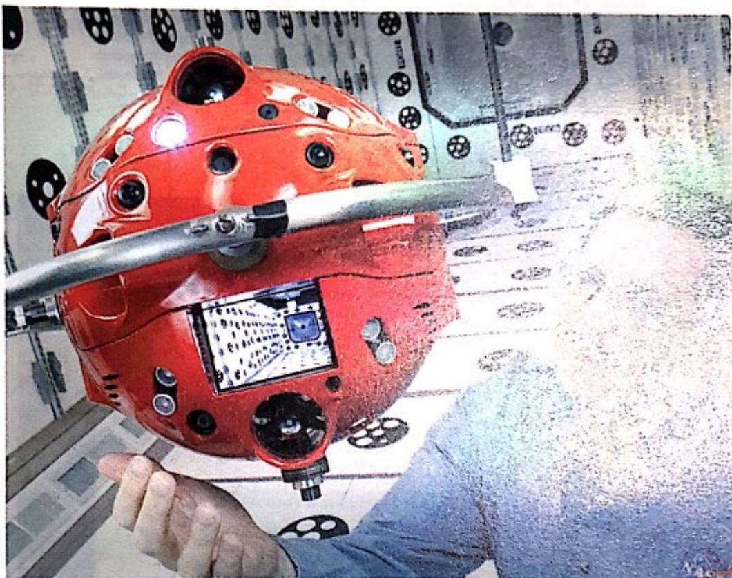
Figure 84 A novel use of the Linux operating system is in the NASA personal satellite assistant, currently under development. The six-inch sphere will float around the International Space Station and act as an environmental monitor and communications device. Its design was inspired by the light saber training droid used by Luke Skywalker in the movie Star Wars .
