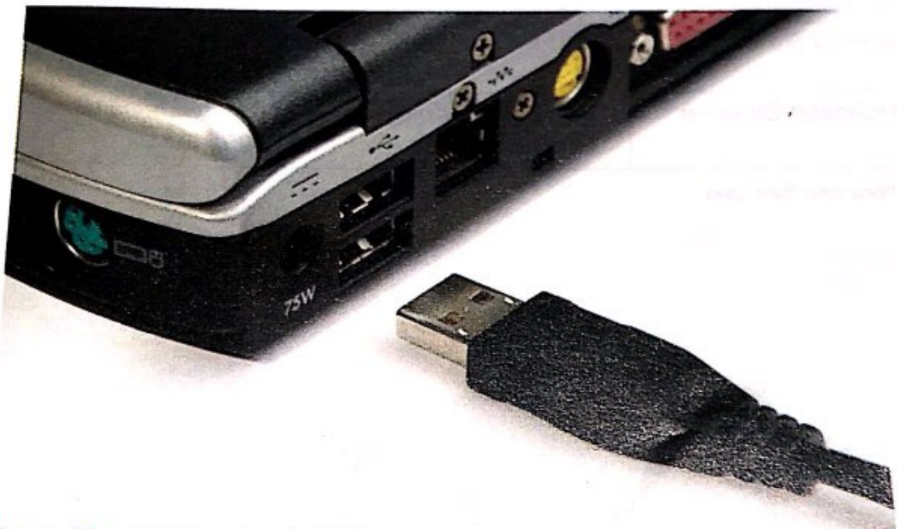
Figure 61 A USB port and a USB connector.
