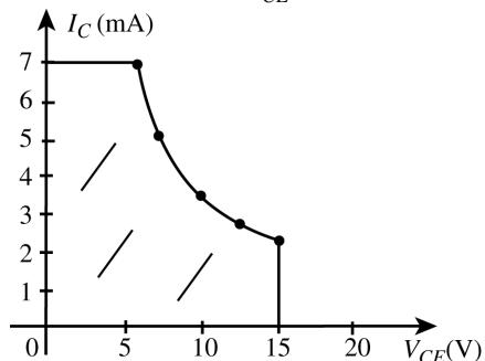
29.  $I_C = I_{C_{\max}}, V_{CE} = \frac{P_{C_{\max}}}{I_{C_{\max}}} = \frac{42 \text{ mW}}{7 \text{ mA}} = 6 \text{ V}$
