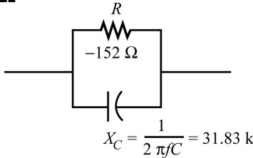
$$Z_T = \frac{(152 \Omega \angle 180^\circ)(31.83 \text{ k}\Omega \angle -90^\circ)}{-152 \Omega - j31.83 \text{ k}\Omega}$$
