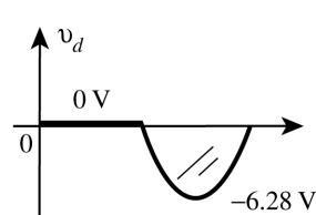
$$I_m = \frac{V_m}{R} = \frac{6.28 \text{ V}}{2 \text{ k}\Omega} = \mathbf{3.14 \text{ mA}}$$
