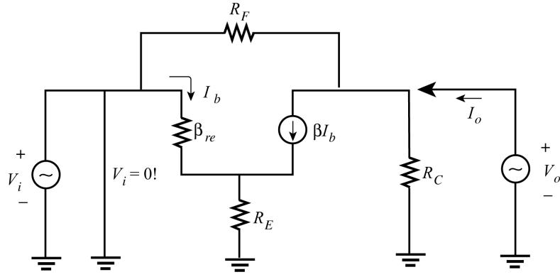
$$V_i = I_b \beta r_e + (\beta + 1) I_b R_E$$
