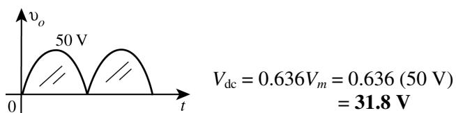
$$V_{dc} = 0.636V_m = 0.636(50 \text{ V}) = 31.8 \text{ V}$$
