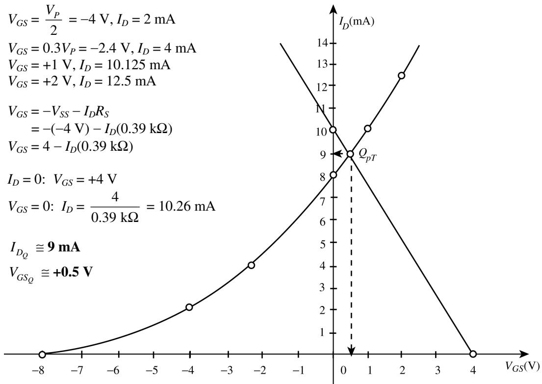
$$(b) V_{DS} = V_{DD} - I_D(R_D + R_S) + V_{SS}$$
