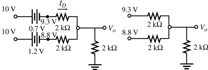
$$\text{Superposition: } V_{o_1}(9.3 \text{ V}) = \frac{1 \text{ k}\Omega(9.3 \text{ V})}{1 \text{ k}\Omega + 2 \text{ k}\Omega} = 3.1 \text{ V}$$
