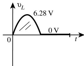
$$I_{L_{\max}} = \frac{6.28 \text{ V}}{10 \text{ k}\Omega} = \mathbf{0.628 \text{ mA}}$$
