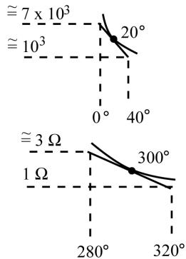
$$\frac{\Delta R}{\Delta T} = \frac{(7000 - 1000) \Omega}{(40 - 0)^\circ C} = \frac{6000 \Omega}{40^\circ C} = 150 \Omega/\text{ }^\circ C$$
