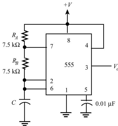
$$f = \frac{1.44}{(R_A + 2R_B)C} = 350 \text{ kHz}$$
