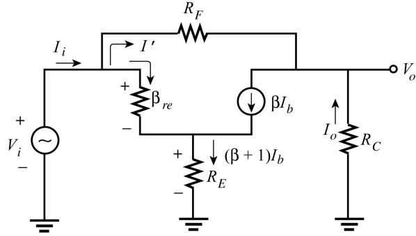
$$(a) A_v: V_i = I_b \beta r_e + (\beta + 1) I_b R_E$$
