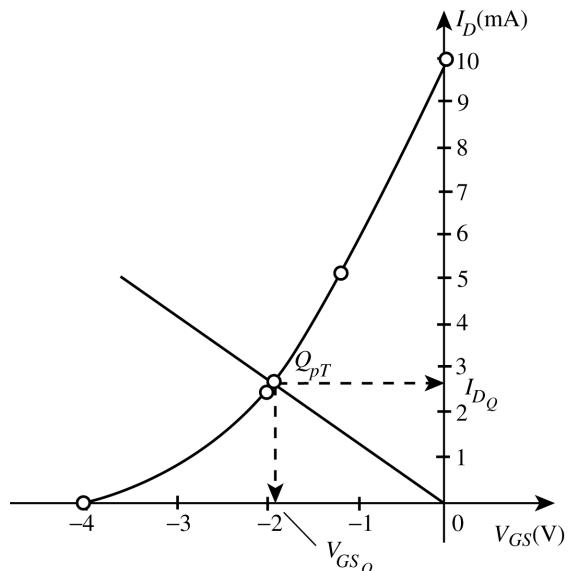
$$7. \quad I_D = I_{DSS}(1 - V_{GS}/V_P)^2 = I_{DSS} \left(1 + \frac{2I_D R_S}{V_P} + \frac{I_D^2 R_S^2}{V_P^2}\right)$$
