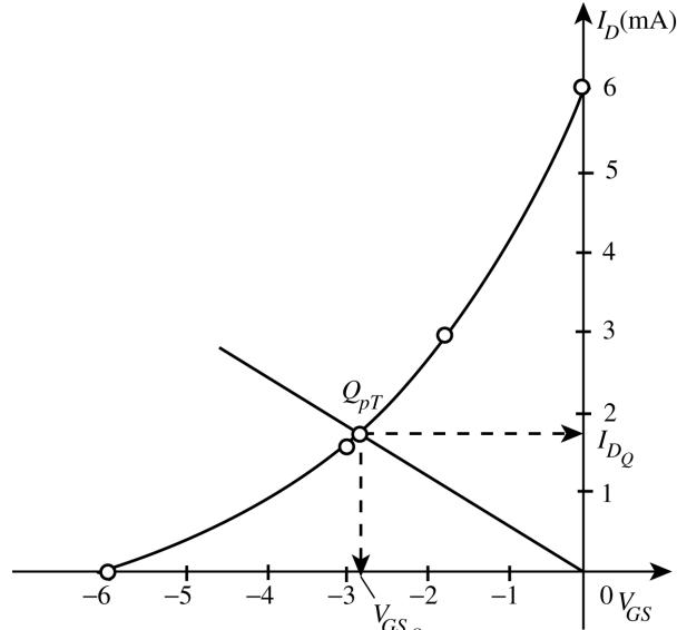
$$9. \quad (a) \quad I_{D_Q} = I_S = \frac{V_S}{R_S} = \frac{1.7 \text{ V}}{0.51 \text{ k}\Omega} = 3.33 \text{ mA}$$
