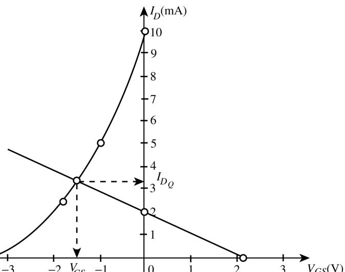
13. (a)  $I_D = I_{DSS} = 10 \text{ mA}$ ,  $V_P = -3.5 \text{ V}$        $V_{GS} = 0 \text{ V}$ ,  $I_D = I_{DSS} = 10 \text{ mA}$        $V_{GS} = V_P = -3.5 \text{ V}$ ,  $I_D = 0 \text{ mA}$
