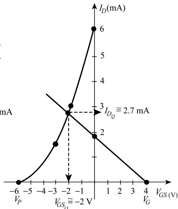
(b)  $V_{DS} = V_{DD} + V_{SS} - I_D(R_D + R_S)$
