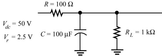
$$\begin{aligned} X_C &= \frac{1.3}{C} = \frac{1.3}{100} = 13 \Omega \\ V'_r &= \frac{X_C}{R} V_r = \frac{13}{100} (2.5 \text{ V}) \\ &= \mathbf{0.325 \text{ V, rms}} \end{aligned}$$
