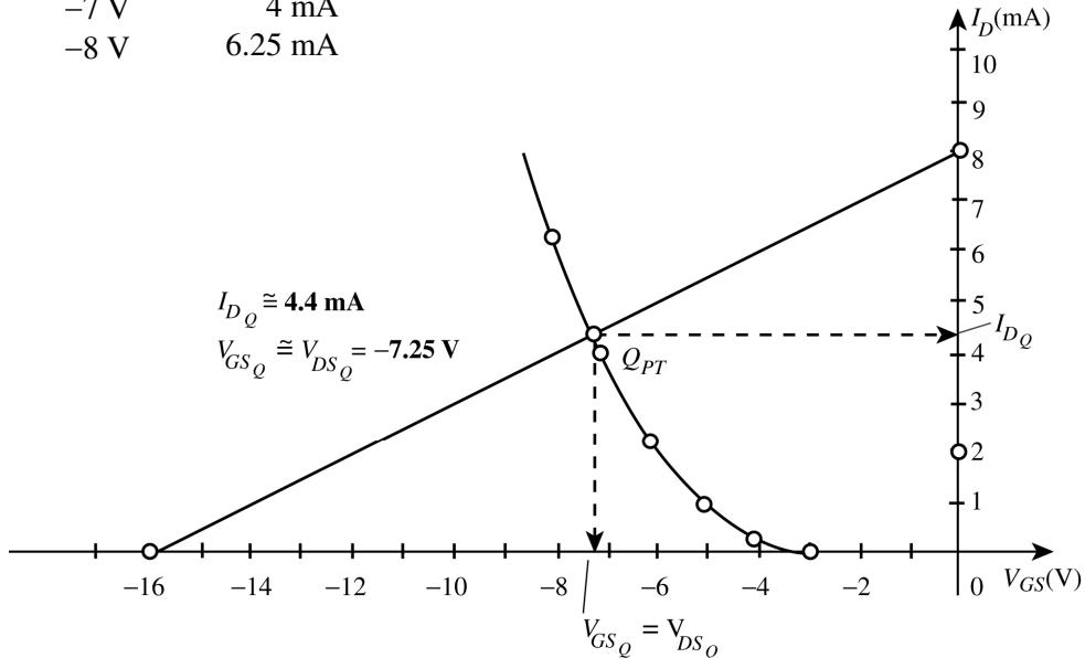
(b)  $V_{DS} = V_{GS} = -7.25 \text{ V}$
