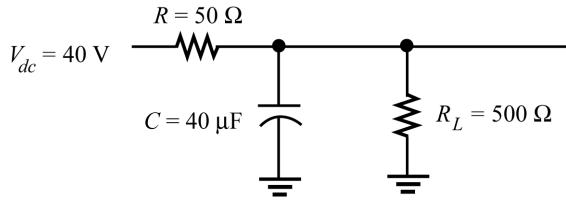
$$\begin{aligned} V'_{dc} &= \frac{R_L}{R + R_L} V_{dc} \\ &= \frac{500}{50 + 500} (40 \text{ V}) \\ &= 36.4 \text{ V} \\ I_{dc} &= \frac{V'_{dc}}{R_L} = \frac{36.4 \text{ V}}{500 \Omega} = \mathbf{72.8 \text{ mA}} \end{aligned}$$
