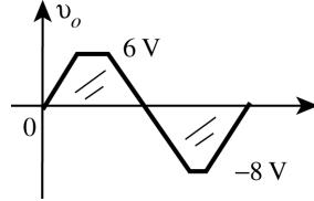
$i_R$ : For  $-8 \text{ V} < v_i < 6 \text{ V}$  there is no conduction through the  $10 \text{ k}\Omega$  resistor due to the lack of a complete circuit. Therefore,  $i_R = 0$  mA.
