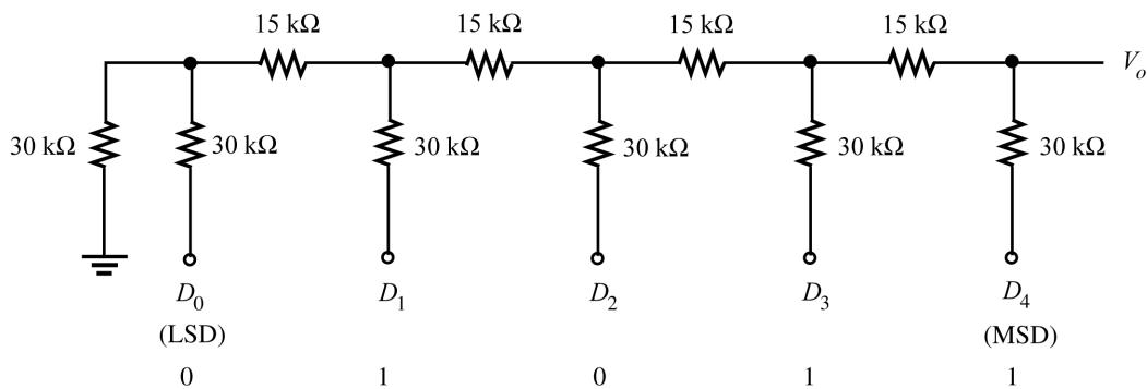
9.  $\frac{11010}{2^5} (16 \text{ V}) = \frac{26}{32} (16 \text{ V}) = 13 \text{ V}$
