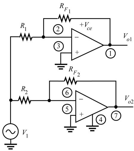
$$V_{o1} = -\frac{R_{F1}}{R_1} V_1 = -\frac{150 \text{ k}\Omega}{R_1} V_1$$
