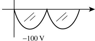
$$I_{\max} = \frac{100 \text{ V}}{2.2 \text{ k}\Omega} = 45.45 \text{ mA}$$
