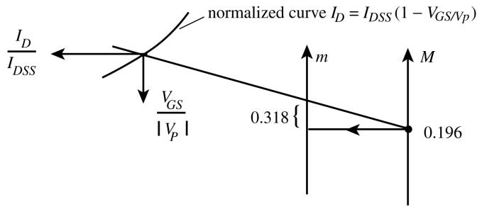
Continue the line until it intersects the  $I_D = I_{DSS}(1 - V_{GS}/V_p)^2$  curve. At the intersection move horizontally to obtain the  $I_D/I_{DSS}$  ratio and move down vertically to obtain the  $V_{GS}/|V_p|$  ratio.
