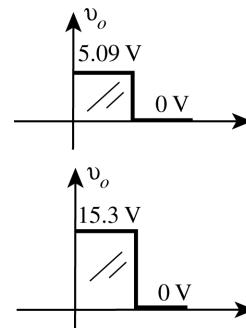
34. (a) For  $v_i = 20$  V the diode is reverse-biased and  $v_o = \mathbf{0 \text{ V}}$ .
