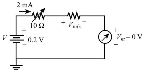
$$\begin{aligned} V &= IR + IR_{\text{unk}} + V_m \\ V &= I(R + R_{\text{unk}}) + 0 \text{ V} \\ R_{\text{unk}} &= \frac{V}{I} - R \\ &= \frac{0.2 \text{ V}}{2 \text{ mA}} - 10 \Omega \\ &= 100 \Omega - 10 \Omega \\ &= 90 \Omega \end{aligned}$$
