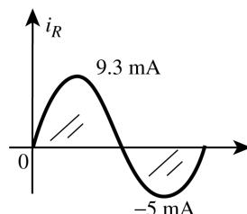
$$I_{\max(\text{reverse})} = \frac{10 \text{ V}}{1 \text{ k}\Omega + 1 \text{ k}\Omega} = 0.5 \text{ mA}$$
