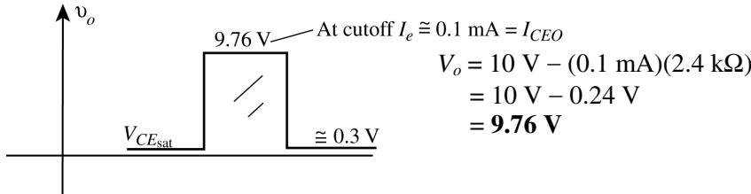
58.  $I_{C_{\text{sat}}} = 8 \text{ mA} = \frac{5 \text{ V}}{R_C}$
