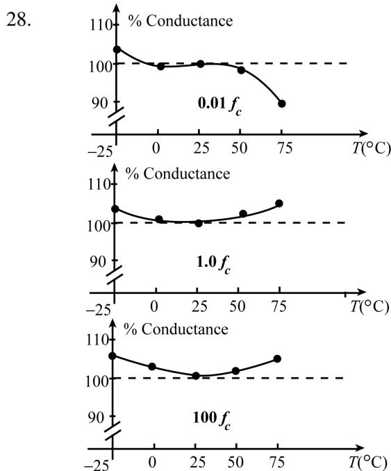
Except for low illumination levels ( $0.01f_c$ ) the % conductance curves appear above the 100% level for the range of temperature. In addition, it is interesting to note that for other than the low illumination levels the % conductance is higher above and below room temperature ( $25^\circ\text{C}$ ). In general, the % conductance level is not adversely affected by temperature for the illumination levels examined.
