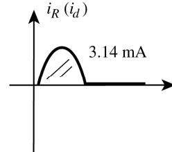
24.  $V_m = \frac{V_{dc}}{0.318} = \frac{2 \text{ V}}{0.318} = \mathbf{6.28 \text{ V}}$
