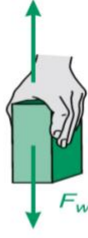
(a) The upward force of the hand equals the downward force of the weight.
