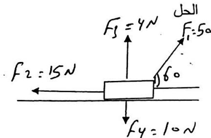
\* A box moves horizontally frictionless in right direction with displacement  $d = 5 \text{ m}$  as shown in the figure What is the total work done
