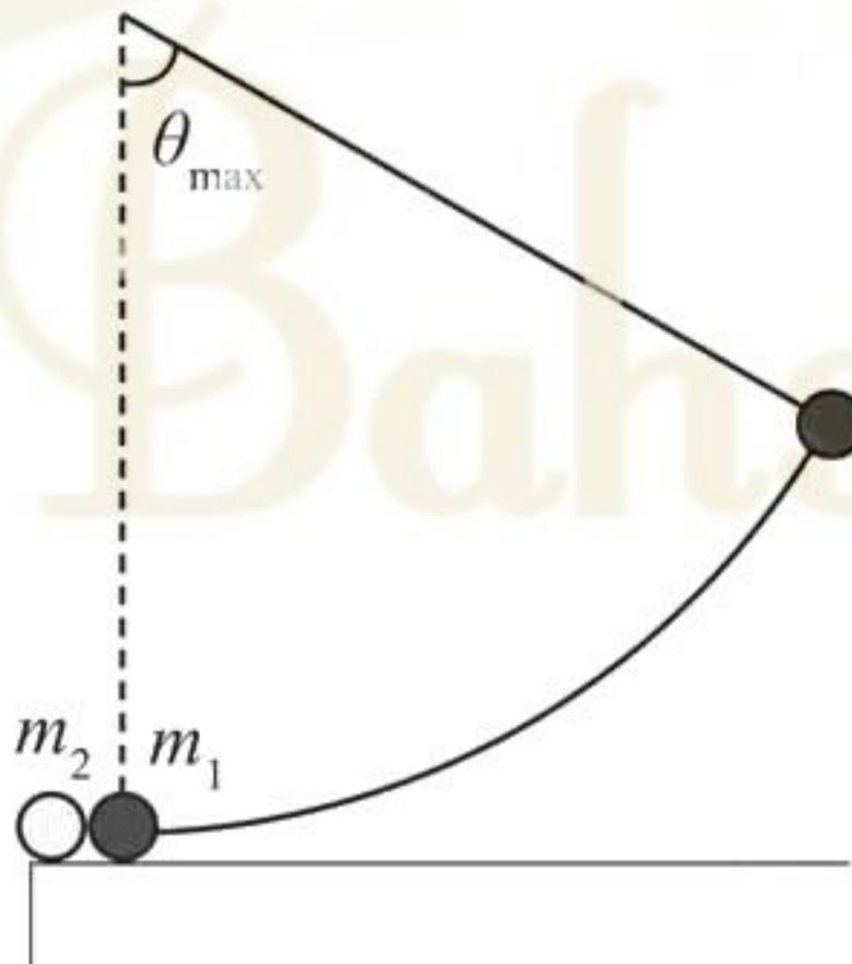
$$\frac{1}{2}m_1v_1^2 + \frac{1}{2}m_2v_2^2 = \frac{1}{2}m_1v'_1^2 + \frac{1}{2}m_2v'_2^2$$
