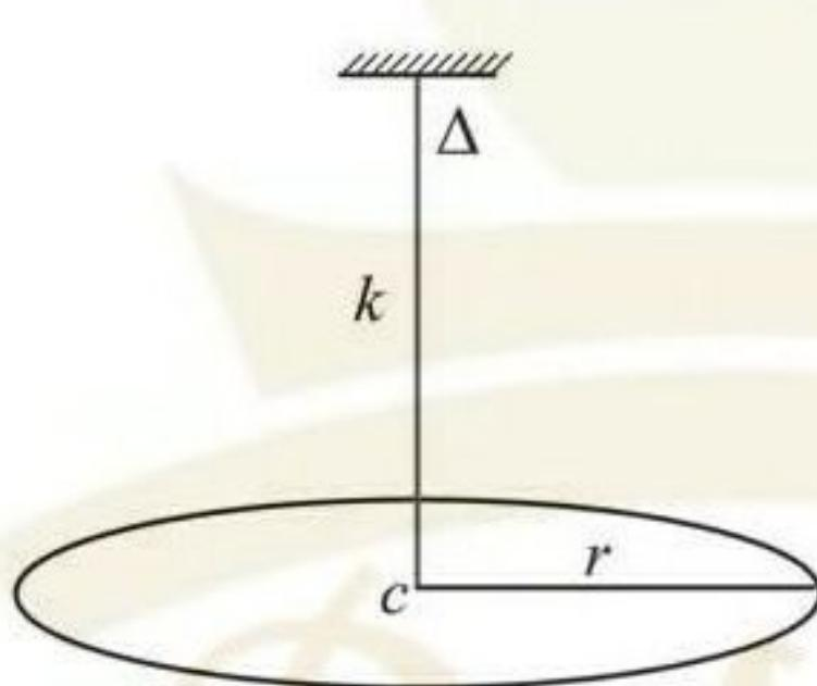
$$\omega_0 = \frac{2\pi}{T_0} = \frac{2\pi}{2} = \pi rad.s^{-1} , X_{\max}, \omega_0, \varphi, \theta_{\max} \\ t=0 \\ \theta = +\pi \quad \left. \theta = \theta_{\max} \cos(\omega_0 t + \varphi) \right|_{t=0} + \pi = \theta_{\max} \cos \varphi ..... (1)$$
