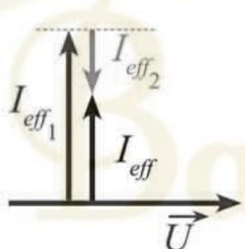
$$\vec{I}_{eff} = \vec{I}_{effL} + \vec{I}_{effc} \Rightarrow I_{eff} = I_{effc} - I_{effL} = 10 - 2.5 = 7.5 A \quad (3)$$
