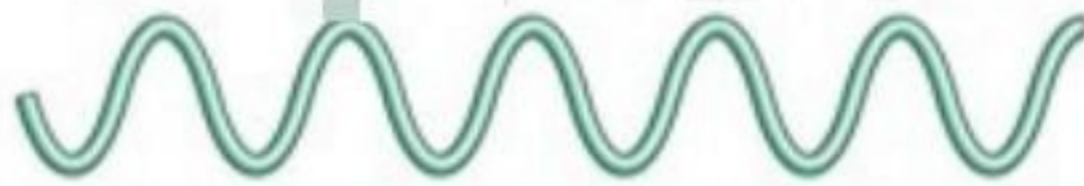
(b) Spring stretched near its elastic limit
