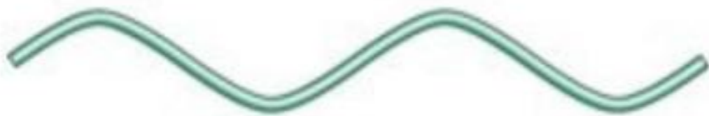
(c) Spring stretched beyond its elastic limit
