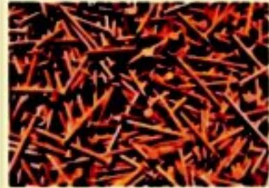
Fig (3-10) Rusty nails after exposure to moisture
