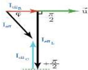
$$I_{eff}^2 = I_{effR}^2 + (I_{effL} - I_{effC})^2$$
