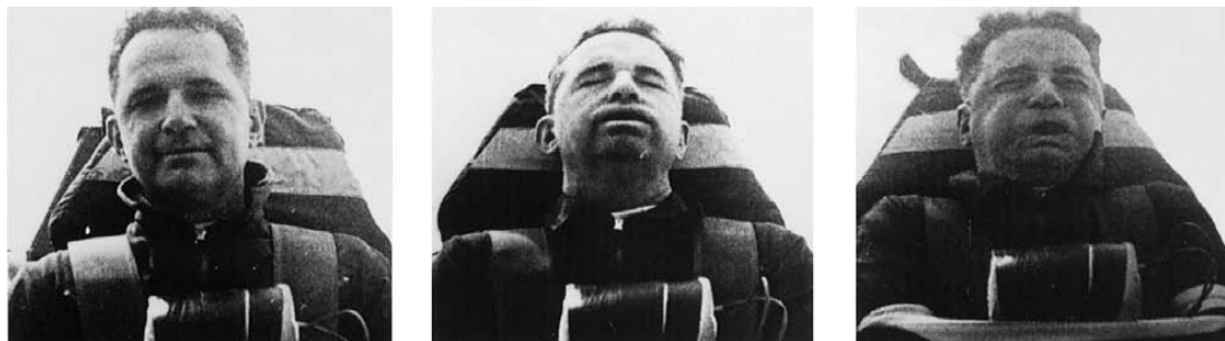
Fig. 2-7 Colonel J. P. Stapp in a rocket sled as it is brought up to high speed (acceleration out of the page) and then very rapidly braked (acceleration into the page). (Courtesy U.S. Air Force)
