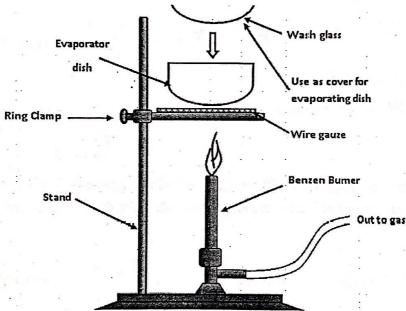
8. Cover the evaporating dish with the watch glass and place it on the wire gauze.
