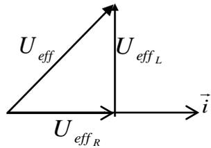
$\vec{U}_{eff} = \vec{U}_{effR} + \vec{U}_{effL}$ $U_{eff}^2 = U_{effR}^2 + U_{effL}^2$ |
