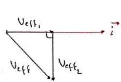
$$V_{eff}^2 = V_{eff,1}^2 + V_{eff,2}^2$$
