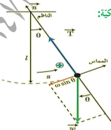
$$\omega_0 = \frac{2\pi}{T_0} = \sqrt{\frac{mgd}{I_{\Delta}}} \Rightarrow T_0 = 2\pi \sqrt{\frac{I_{\Delta}}{mgd}}$$
