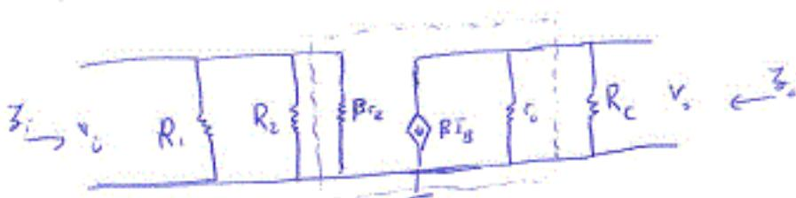
$$Z_i = R_1 \parallel R_2 \parallel \beta r_e$$
