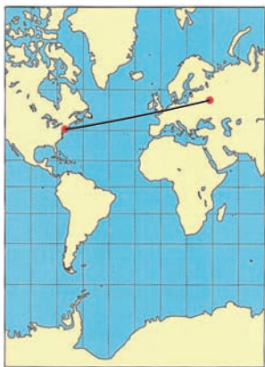
▲ Figure 7.3.2 A flight path with constant compass heading from New York City to Moscow follows a spiral toward the North Pole but is a straight line segment on a Mercator projection.
