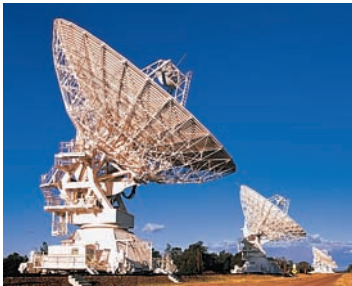
John Mead/Science Photo Library/Photo Researchers Incoming signals are reflected by the parabolic antenna to the receiver at the focus.
