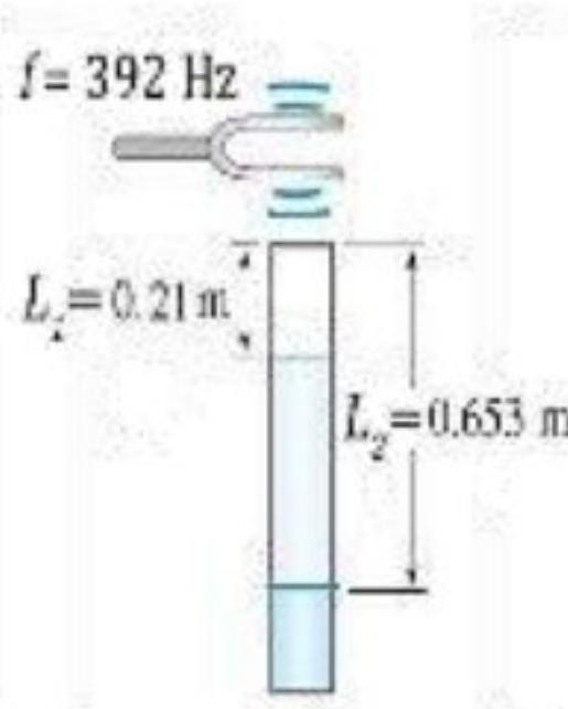
$$\Delta L = L_2 - L_1 = \frac{\lambda}{2} \Rightarrow 0.653 - 0.21 = \frac{\lambda}{2} \Rightarrow \lambda = 0.886 \text{ m} \quad \text{الحل:}$$
