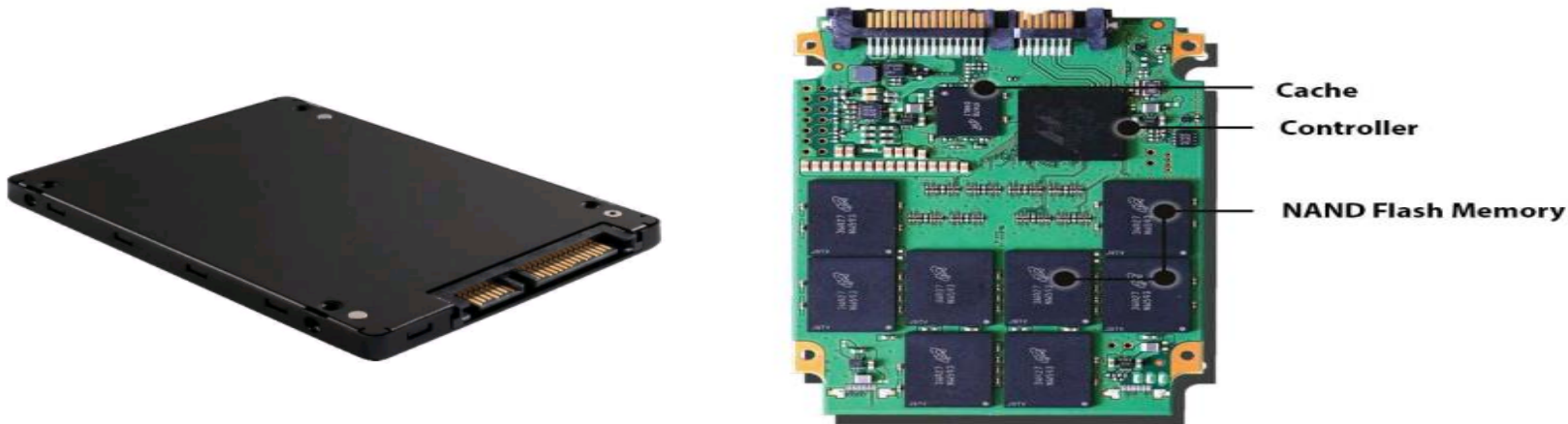
Figure 1-9 Solid State Drive and its internal circuitry showing NAND flash.
