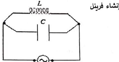
$$U_{eff} = X_C I_{eff_c} \quad : I_{eff_c} \text{ نحسب}$$
