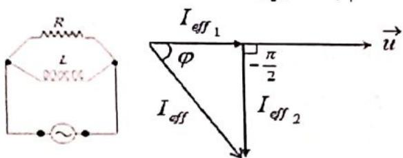
$$\overrightarrow{I_{\text{eff}}} = \overrightarrow{I_{\text{eff}_1}} + \overrightarrow{I_{\text{eff}_2}}$$
