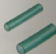
(b) Doubling the radius more than doubles the cross-sectional area.
