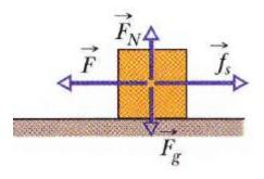
• If the body does sliding, the fractional force is a kinetic fractional force  $f_k$ .
