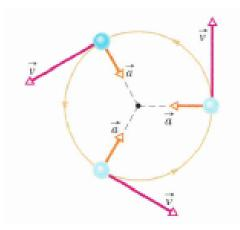
• The vector quantities of acceleration and force are directed toward the centre of curvature of the particle's path.
