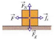
• The fractional force is parallel to the surface and directed so as to oppose the sliding.
