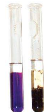
Hexane does not react with purple \text{KMnO}_4 (left); cyclohexene (right) reacts, producing a brown-black precipitate of \text{MnO}_2 .
