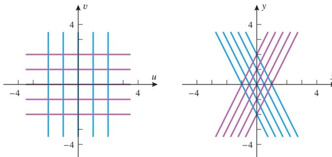
**Solution (d).** The image of a region can often be found by finding the image of its boundary. In this case the images of the boundary lines  $u = -2$ ,  $u = 2$ ,  $v = -2$ , and  $v = 2$  enclose the diamond-shaped region in the  $xy$ -plane shown in Figure 14.7.4. ◀
