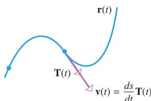
The length of the velocity vector is the speed of the particle, and the direction of the velocity vector is the direction of motion.
