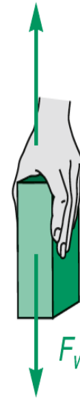
(a) The upward force of the hand equals the downward force of the weight.
