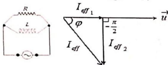
$$\overrightarrow{I_{\text{eff}}} = \overrightarrow{I_{\text{eff}_1}} + \overrightarrow{I_{\text{eff}_2}}$$
