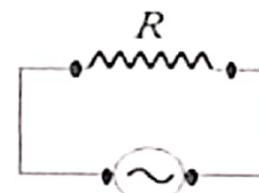
$$\bar{i} = I_{\max} \cos(\omega t + \bar{\varphi}_1)$$
