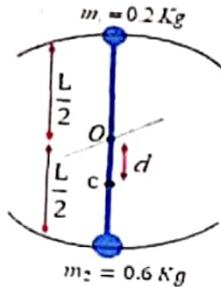
$$T_0 = 2\pi \sqrt{\frac{I_\Delta}{m g d}} \dots (1)$$
