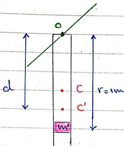
$$T_0 = 2\pi \sqrt{\frac{I_D}{mgd}} \quad (1)$$
