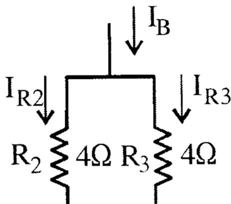
$$I_{R_2} = I_{R_3} = \frac{I_B}{2} = \frac{1A}{2} = 0.5A$$
