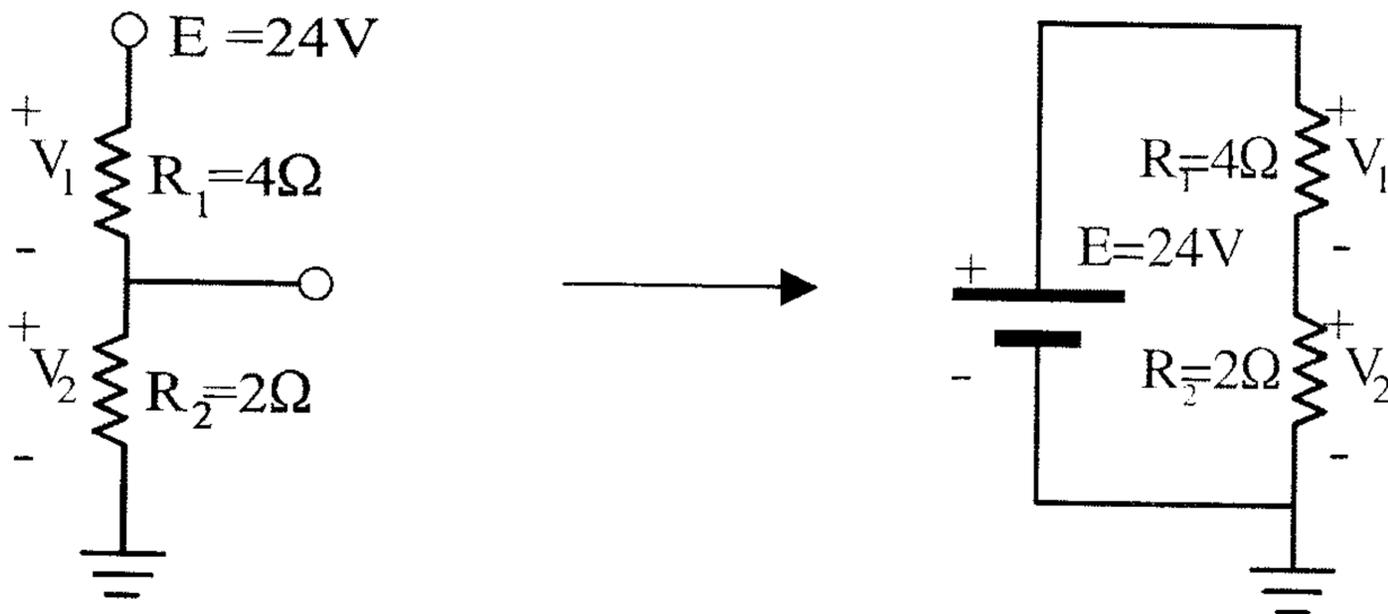
$$V_2 = \frac{E R_1}{R_1 + R_2} = \frac{(24V)(2\Omega)}{4\Omega + 2\Omega} = 8V, \quad V_1 = \frac{E R_2}{R_1 + R_2} = \frac{(24V)(4\Omega)}{4\Omega + 2\Omega} = 16V$$
