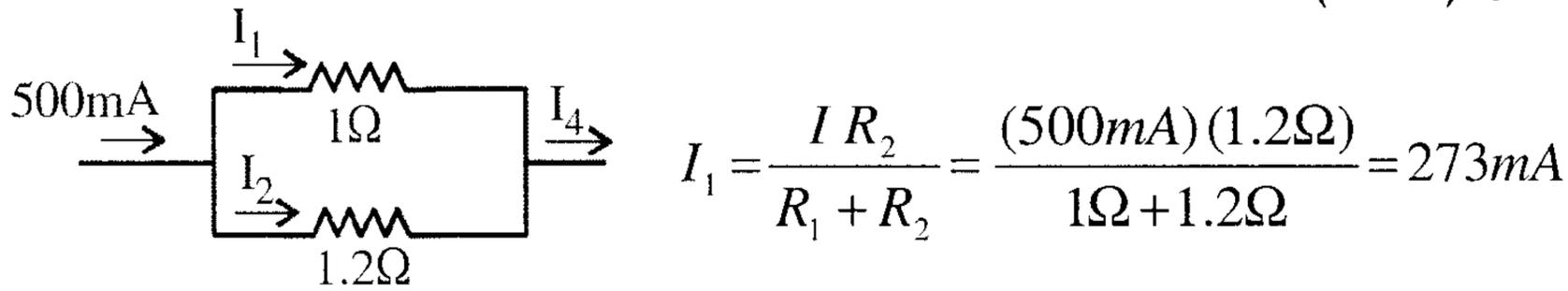
$$I_2 = \frac{I R_1}{R_1 + R_2} = \frac{(500mA)(1\Omega)}{1\Omega + 1.2\Omega} = 227mA$$
