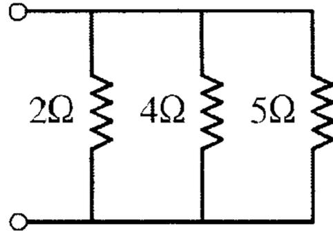
$$\frac{1}{R_T} = \frac{1}{R_1} + \frac{1}{R_2} + \frac{1}{R_3} = \frac{1}{2\Omega} + \frac{1}{4\Omega} + \frac{1}{5\Omega} = \frac{19}{20}$$
