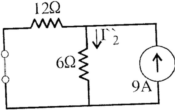
$$I_2'' = \frac{(9A)(12\Omega)}{6\Omega + 12\Omega} = \frac{108A\Omega}{18\Omega} = 6A$$
