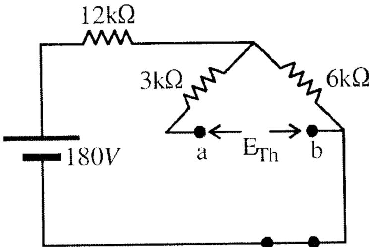
$$E_{Th} = \frac{(180V)(6k\Omega)}{6k\Omega + 12k\Omega} = \frac{1080}{18} = 60V$$
