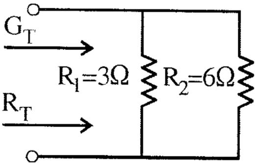
$$\frac{1}{R_T} = \frac{1}{R_1} + \frac{1}{R_2} = \frac{1}{3\Omega} + \frac{1}{6\Omega} = \frac{3}{6\Omega}$$
