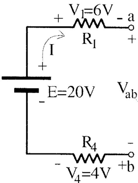
$$+ E - V_1 - V_{ab} - V_4 = 0$$
