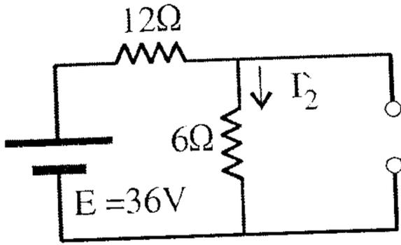
$$I_2' = \frac{E}{R_T} = \frac{36V}{12\Omega + 6\Omega} = \frac{36V}{18\Omega} = 2A$$
