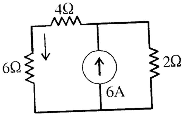
$$I_{6\Omega}''' = \frac{(6A)(2\Omega)}{12\Omega} = \frac{12}{12\Omega} = 1A \quad \downarrow$$
