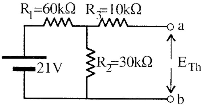
$$E_{Th} = \frac{R_2 E}{R_1 + R_2}$$
