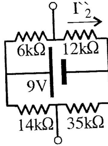
$$I_2'' = \frac{(9V)}{6k\Omega + 12k\Omega} = \frac{9V}{18k\Omega} = 0.5mA$$
