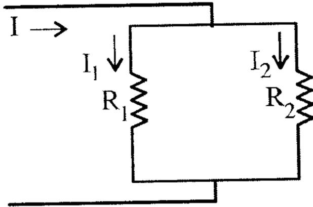
$$R_T = \frac{R_1 R_2}{R_1 + R_2}$$
