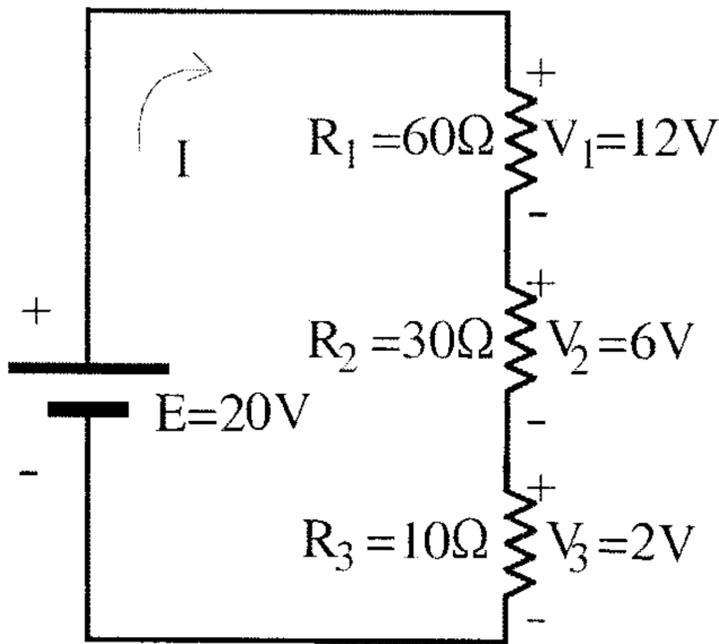
$$V_1 = \frac{E}{R_T} \cdot R_1 = \frac{20 \times 60}{100} = 12V$$
