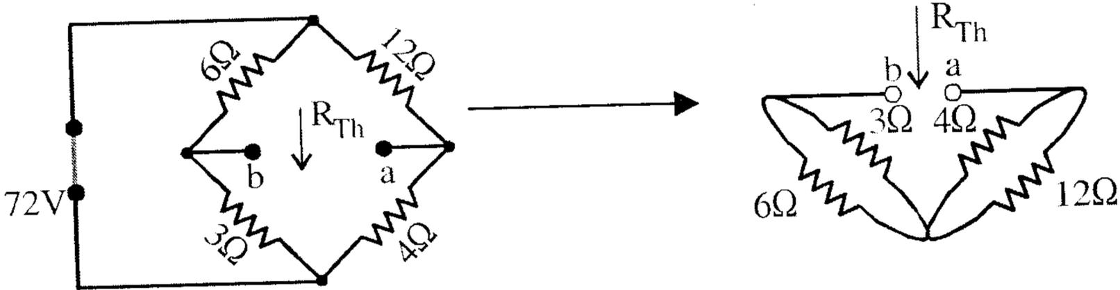
$$V_{6\Omega} = \frac{(6\Omega)(72V)}{6\Omega + 3\Omega} = \frac{432}{9} = 48V$$
