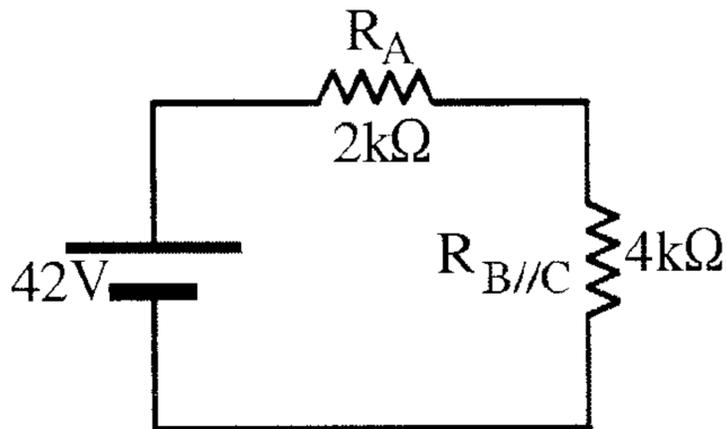
$$\begin{aligned} \therefore R_T &= R_A + R_{B//C} \\ &= 2k\Omega + 4k\Omega \end{aligned}$$
