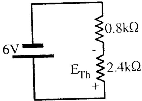
$$E_{Th} = \frac{(6V)(2.4k\Omega)}{2.4k\Omega + 0.8k\Omega} = \frac{14.4}{3.2} = 4.5V$$
