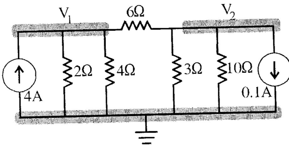
$$\left(\frac{1}{2} + \frac{1}{4} + \frac{1}{6}\right)V_1 - \frac{1}{6}V_2 = 4$$
