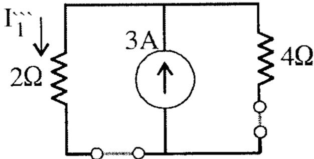
$$I_1''' = \frac{(3A)(4\Omega)}{2\Omega + 4\Omega} = \frac{12A}{6\Omega} = 2A$$
