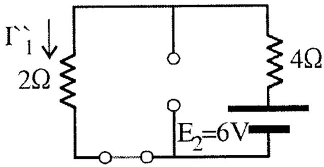
$$I_1'' = \frac{(6V)}{2\Omega + 4\Omega} = \frac{6V}{6\Omega} = 1A$$
