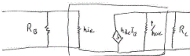
$$Z_i = R_B \parallel h_{ie} = \frac{(330k)(1.17k)}{(330k) + (1.17k)} = 1165.87 \Omega$$
