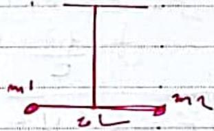
$$\frac{T_0'}{T_0} = \sqrt{\frac{I_D'}{I_D}}$$
