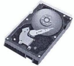
Hard disks are capable of storing vast amounts of data in multiple gigabytes. Hard disk speeds vary – the faster the speed of your hard disk, the faster it will store or retrieve data. It is wise to “defragment” your hard disk occasionally, to enable it to easily locate and unite parts of files, and therefore speed up work on your computer. Additional hard disk memory makes an affordable way of upgrading your computer.
