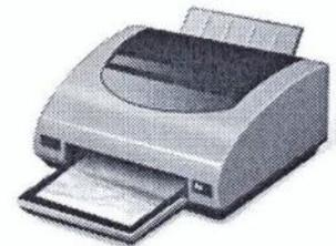
A **laser printer** is a high-speed printer that uses a laser beam to form high quality images on a page. You can buy either a black-and-white or colour laser printer.
