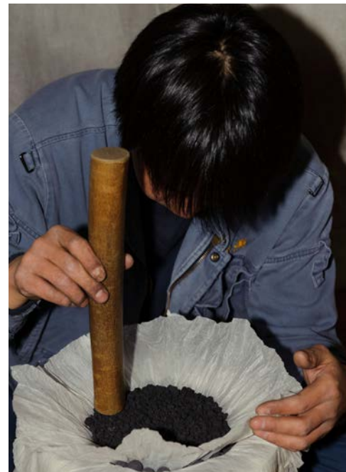
Loading shells with black powder
