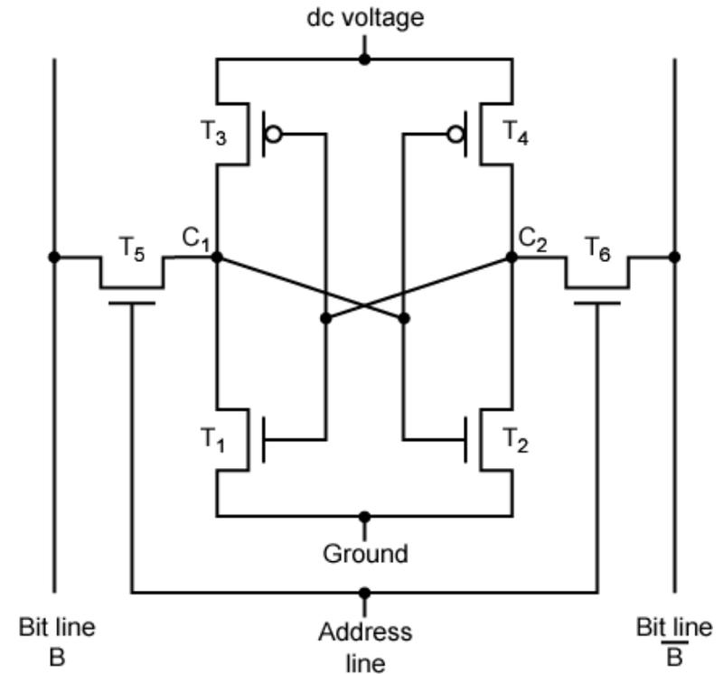
For a write operation, the desired bit value is applied to line  $B$  &  $\bar{B}$ . This forces  $T_1, T_2, T_3, T_4$  into the proper state.
