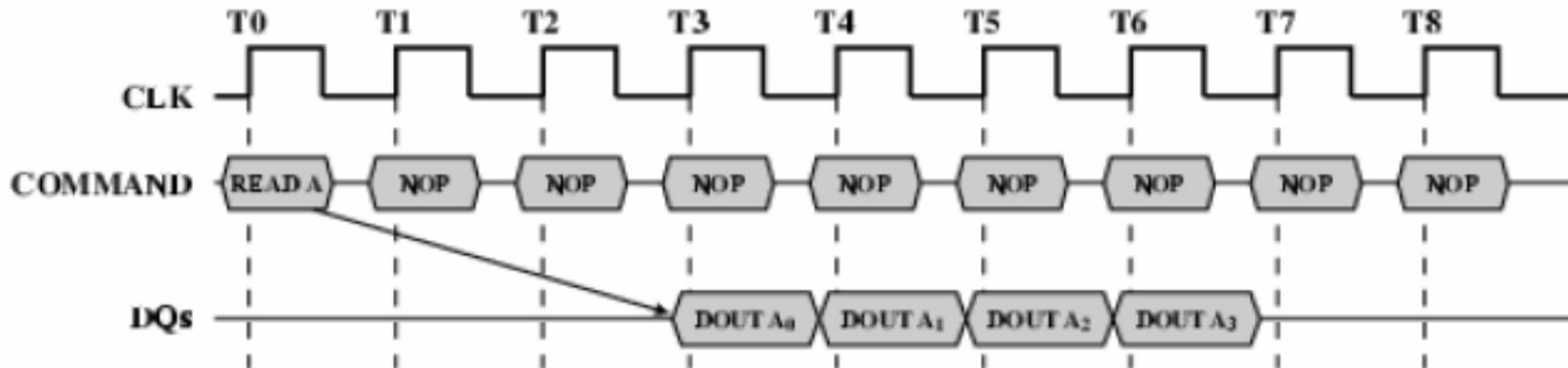
Figure 5.13. SDRAM read timing (burst length = 4 &  $\overline{CAS}$  latency = 2
