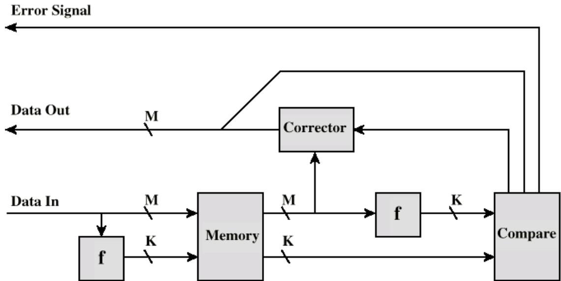
Code is used to detect and possibly correct errors. A new set of  $k$  code is generated from  $k$  data bits and compared with fetched code bits. This yields to:
