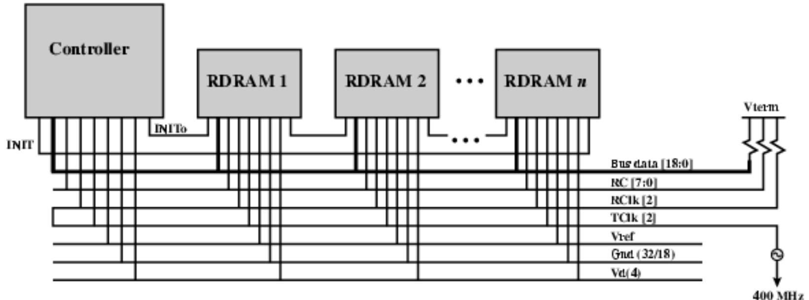
A controller connects a # of RDRAM module via a common bus. The bus includes 18 data lines (16 actual data & 2 parity) cycling at twice the clock rate; 1 bit is sent at the leading and following edge of each clock cycle
