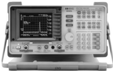
FIG. 25.8 Spectrum analyzer. (Courtesy of Hewlett Packard)
