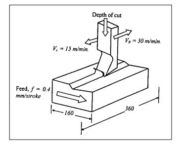
16. Comment on the set-up shown at Fig. 7.13, listing any faults in work or tool setting.
