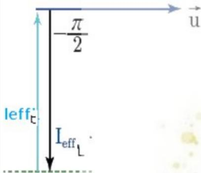
$$\begin{aligned} \vec{I}_{eff} &= \vec{I}_{effL} + \vec{I}_{effC} \\ I_{eff} &= I_{effC} - I_{effL} = 0 \end{aligned}$$
