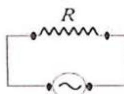
$$\bar{i} = I_{\max} \cos(\omega t + \bar{\varphi}_1)$$
