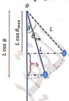
$$\begin{aligned} E_{k_2} &= \bar{W}_{\vec{w}} \\ \frac{1}{2} m v^2 &= m g h \Rightarrow \\ v^2 &= 2 g h \Rightarrow \\ v &= \sqrt{2 g h} \end{aligned}$$
