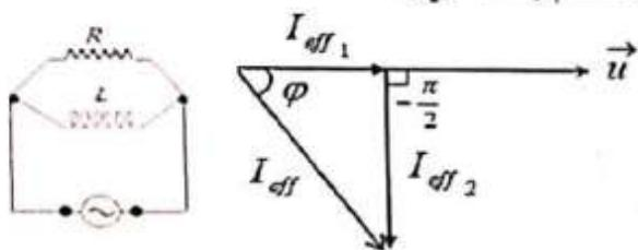
$$\overrightarrow{I_{\text{eff}}} = \overrightarrow{I_{\text{eff}_1}} + \overrightarrow{I_{\text{eff}_2}}$$
