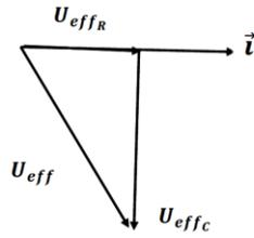
$$U_{eff} = \sqrt{U_{eff_R}^2 + U_{eff_C}^2} = \sqrt{1600 + 900} = \sqrt{2500} = 50\text{V}$$
