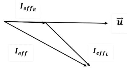
$$I_{eff} = \sqrt{I_{eff_R}^2 + I_{eff_L}^2 + 2I_{eff_R} I_{eff_L} \cos \varphi_L} = \sqrt{16 + 25 + 2 \times 4 \times 5 \times 0.2} = \sqrt{49} = 7\text{A}$$
