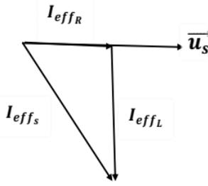
$$I_{eff_s} = \sqrt{I_{eff_R}^2 + I_{eff_L}^2} = \sqrt{16 + 9} = 5 \text{ A}$$
