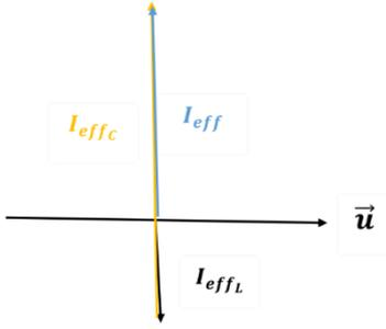
$$I_{eff} = I_{eff_c} - I_{eff_L} = 10 - 2.5 = 7.5A$$
