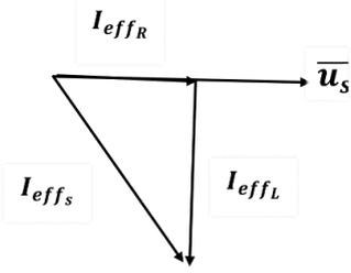
$$I_{eff_L} = \sqrt{I_{eff_s}^2 - I_{eff_R}^2} = \sqrt{25 - 16} = 3A$$
