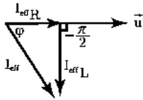
$$I_{eff} = \sqrt{I_{effR}^2 + I_{effL}^2} = \sqrt{16 + 9} = 5 A$$
